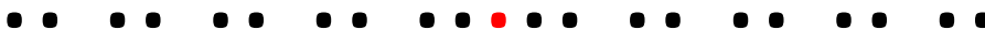
Fig. 6 Images the pattern caused by monochrome light through a slide with multiple slits
